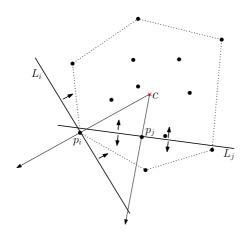
Figure 4: Deciding whether a given point is on the convex hull. The point  $p_i$  is on the convex hull shown by dotted lines since one of the half plane defined by the line  $L_i$  is empty. The point  $p_j$  is not so since none of the half planes is empty.
