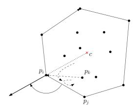
Figure 2: Finding the counter-clockwise next extreme point using a ray from  $p_i$  and the centroid c.
