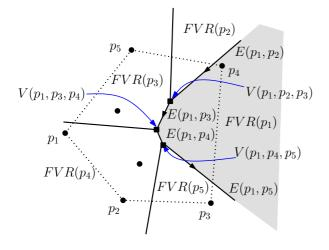
Figure 1: Farthest-point Voronoi diagram. Vertices on the convex hull are  $\{p_1, \ldots, p_5\}$ .  $FVR(p_i)$  and  $E(p_i, p_j)$  are the Voronoi region for point  $p_i$  and Voronoi edge for two points  $p_i$  and  $p_j$ , respectively.
