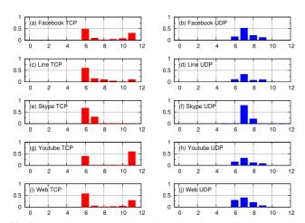
Fig. 3 TCP and UDP packet size distributions for 5 applications (x-axis: bin index, y-axis: PDF).
