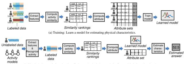
(b) Physical characteristic estimation: Estimate physical characteristics from unlabeled acceleration data. Fig. 1 Overview of our method. (a) Training and (b) Physical characteristic estimation.
