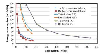
Figure 8 Comparison of energy consumptions for 1-Mbit data transmission and reception for various devices
