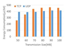
Figure 6 Comparison of energy consumptions for 1-bit transmission with various data transmission sizes
