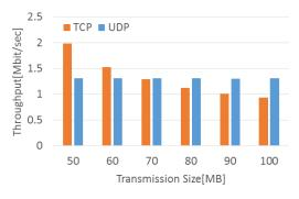
Figure 4 Comparison of throughput characteristics for various data transmission sizes
