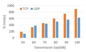
Figure 5 Comparison of transmission times for various data transmission sizes
