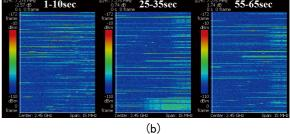
ig. 7 Spectrogram of the microwave oven leakage when heating (a) water and (b) French fries.
