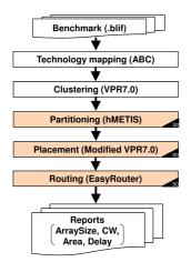
Fig. 5 Design flow of proposed 3D FPGA.
