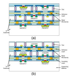
Fig. 1 Cross-sectional structure of 3D LSI architecture: (a) face-up stacking; (b) face-down stacking.
