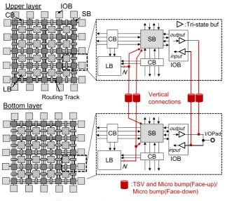
Fig. 4 Proposed 3D routing structure.
