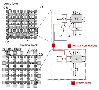
Fig. 3 Functionally distributed 3D architecture with face-down stacking.
