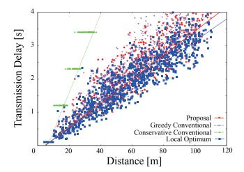
$\boxtimes~9~$  End-to-End Delay in Wireless Multihop Transmissions (  $0.1~{\rm m/s}$  ).
