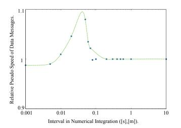
☑ 11 End-to-End Transmission Delay with Various interval in Numerical Integration.
