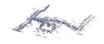
Fig. 8 Example of city-scale 3D reconstruction (April, 2011, Kamaishi, Iwate). This result consists of one thousand omnidirectional images.
