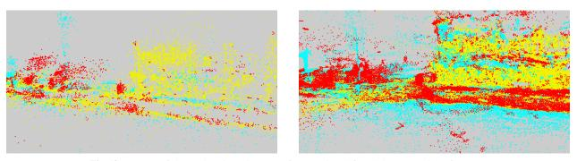
Fig. 10 A scene of change detection using sparse feature points (left) and dense 3D points of PMVS2 (right) comparing April, 2011 and July, 2011, Rikuzentakata, Iwate. Red, blue and yellow show disappearance, appearance and no-change, respectively.
