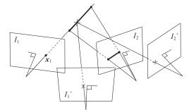
Fig. 15 Geometry of two sets of multi-view perspective images taken at different times. For each pixel  $x_1$  of  $I_1$ , the probability that the scene depth has changed is estimated.
