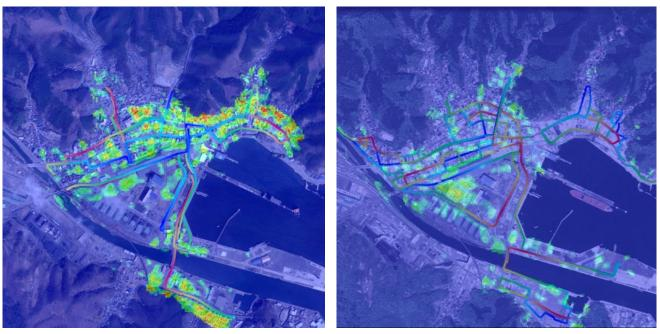
Fig. 26 City-scale Debris Probability in Kamaishi before the recovery operation (Left: April 26th, 2011, Right: August 17th, 2013). Color denotes probability of debris, with blue corresponding to 0 and red to 1.
