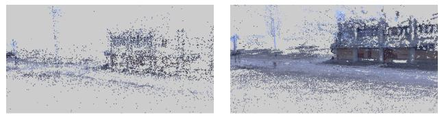
Fig. 9 Example of dense 3D reconstruction scene using sparse feature points (left) and PMVS2 (right) (July, 2011, Rikuzentakata, Iwate).
