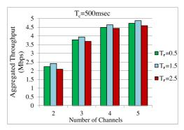
Fig. 7 Comparison of throughput under variation of parameter  $T_r$ .
