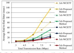
Fig. 18 Comparison of average end-to-end jitter in Scenario 2.
