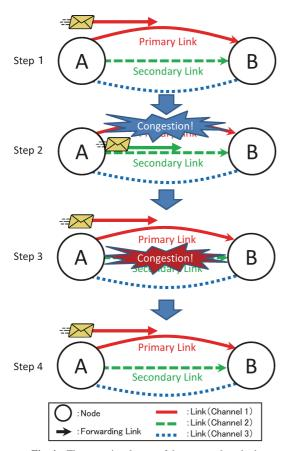
Fig. 4 The operational steps of the proposed method.
