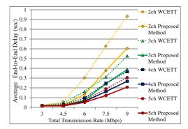
Fig. 17 Comparison of average end-to-end delay in Scenario 2.
