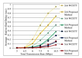
Fig. 13 Comparison of average end-to-end delay in Scenario 1.
