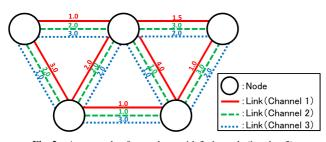
**Fig. 2** An example of a topology with 3 channels (i.e., k = 3).
