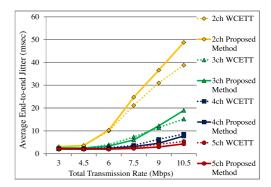
Fig. 14 Comparison of average end-to-end jitter in Scenario 1.
