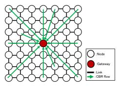
Fig. 6 Network topology in Scenario 2: In this topology, the central node behaves as a gateway, and 48 CBR flows are generated from all nodes (except the gateway) to the gateway.
