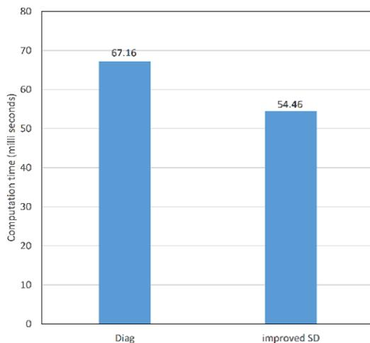
**Fig. 3** A comparison of average runtimes for the deformation of a dragon model. Left: using diagonalization (Diag). Right: using improved spectral decomposition (improved SD) which includes our algorithm for the computation of the eigenvalues.
