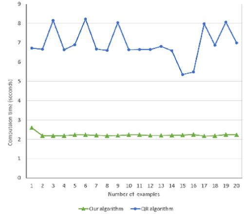
**Fig. 1** Computation time of the eigenvalues of the  $3 \times 3$  real symmetric matrix. Upper: using the QR algorithm. Lower: using our algorithm.
