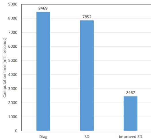
**Fig. 2** A comparison of average runtimes for the computation of the matrix exponential of  $3 \times 3$ . Left: using diagonalization (Diag). Center: using spectral decomposition (SD). Right: using the improved spectral decomposition (improved SD) which includes our algorithm for the computation of the eigenvalues.
