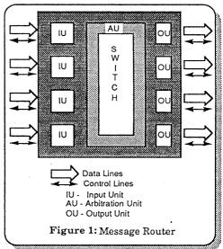
should be as simple as possible, and ensure that deadlock and livelock conditions cannot exist in the network. The arbitration unit controls access to the switch and output unit so as to minimize the average delay experienced by a message in the network. The output unit controls the flow of data across the physical channel separating two routers, or a router and a processing element.
