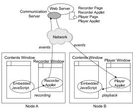
Fig. 8 Implementation of a Web-browser-sharing system based on the recorder and player.
