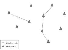
Fig. 2 Example of a system architecture: an ad hoc network consisting of only mobile hosts.
