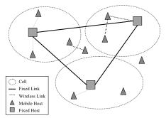
Fig. 1 Example of a system architecture consisting of fixed and mobile hosts.
