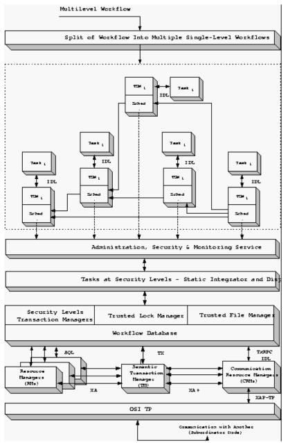
Fig. 4 The MLS distributed workflow architecture.
