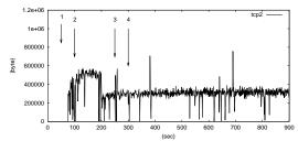
Fig. 12 Traffic pattern of DVTS flow and TCP flow (TCP traffic 2).
