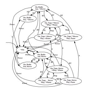
Fig. 4 Global transition system of the Radio/Tape player.
