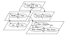
Fig. 3 Hierarchical system specification of the Radio/Tape player.
