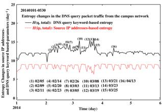
Figure 3 Entropy changes in the total A resource records (RR) based DNS query request packet traffic from the campus network to the top domain DNS (tDNS) server through January 1st to May 30th, 2014. The solid and dotted lines show unique DNS query keywords and the unique source IP addresses based entropies, respectively (day<sup>-1</sup> unit).
