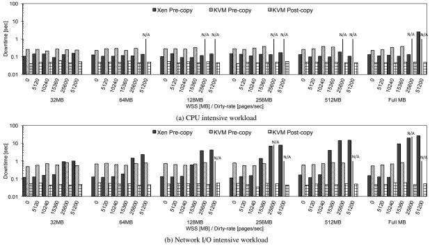
Fig. 2 Downtime caused by each migration method under various workloads. Change the parameter of migrating VM's workload when the collocating VMs run CPU intensive workload (a) and network I/O intensive workload (b).
