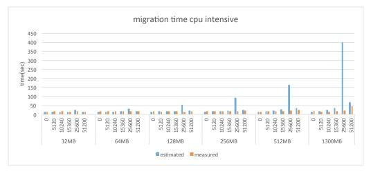
Fig. 6 Comparison of estimated and measured migration time of Xen pre-copy.
