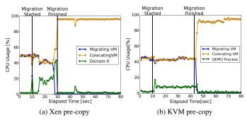
Fig. 1 CPU utilization of each VM on the source host (workload of migrating VM set working set size (WSS): 64 MB, Dirty-rate: 15360 pages/sec). Two VMs (migrating VM and collocating VM) running on the source cause CPU resource contention, and thus live migration starts moving migrating VM at 10 seconds to mitigate the contention.
