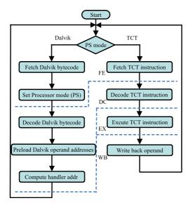
Fig. 4 Behavior of the proposed processor architectural framework.
