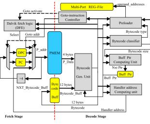
Fig. 8 Block diagram of Dalvik hardware extension.
