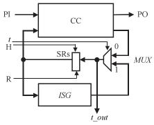
Fig. 4 Model of a synthesized sequential circuit of FSM with DFT.
