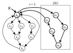
Fig. 3 Example of FSM with DFT.
