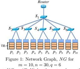
Let NG = (E, N) be the network graph for our framework where E is the set of edges represent VM dependencies and  $N = P \cup S$  is the set of physical machines and switches (Figure: 1). Let  $\mathcal{G} = (V, E, w)$  be the weighted cost graph where  $w : E \to R$  is a function that assigns each edge a weight of traffic cost between two VMs that is a real number.
