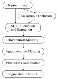
Fig. 1 Block diagram of the segmentation procedure.
