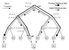
Fig. 12 SMM-A Proc. of handover of source: The S is moving to B5 cell. The S sends Move message to current SP (B4) by way of B5, N6, N3, N1, N2, N5 and B4. N3, N1, N2 and N5 already has MFCE for G, then, they create another MFCE with 'transition' flag;  $E'_{G}(N3) = \{-1, 1, -1\}, E'_{G}(N1) = \{0, -1, 1\}, E'_{G}(N2) = \{1, -1, -1\}, and E'_{G}(N5) = \{1, 0, -1\}.$  When the S has moved to B5 cell, it sends Complete message. N3, N1, N2 and N5 remove older MFCFs and clear the 'transition' flag.
