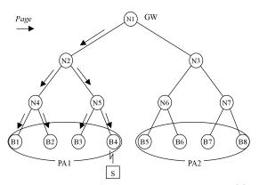
Fig. 8 SMM-A Proc. of forming RPT and SPT (1): The S is at PA1 and N1 has a paging cache. N1 sends Page message to N2. N2, N4 and N5 forward the Page to all downstream interfaces. B1-B4 broadcast the Page via an air interface.
