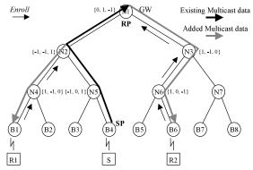
Fig. 10 SMM-A Proc. of forming RPT and SPT (3): R1 and R2 are at B1 and B6 cells, respectively. They send *Enroll* message to N1. N4, N6 and N3 have no MFCE for G, then, they create  $E_{\rm G}({\rm N4}) = \{1, -1, 0\}, E_{\rm G}({\rm N6}) = \{1, 0, -1\}$ and  $E_{\rm G}({\rm N3}) = \{1, -1, 0\}$ . N2 already has MFCE for G, then, it update to  $E_{\rm G}({\rm N2}) = \{-1, -1, 1\}$ .
