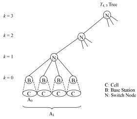
**Fig. 16** Tree model: v-ary tree of depth  $\mu$ ;  $T_{v,\mu}$ .
