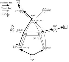
Fig. 14 SMM-C Proc. of source handover (2): The S is moving to the access network attached to N6. The S sends Launch message to the new GW, i.e., N6. N6 reports to the BSN that it becomes the SP for G and sets up a tunnel to N5 through which encapsulated multicast packets are forwarded by unicasting.
