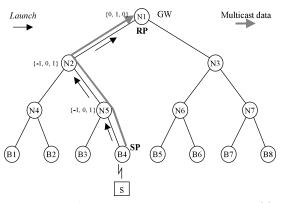
Fig. 9 SMM-A Proc. of forming RPT and SPT (2): Now, the S is at B4 cell and sends *Launch* message to N1 to set up a path from the S to RP (N1).  $E_{\rm G}(\rm N5) = \{-1,0,1\}, E_{\rm G}(\rm N2) = \{-1,0,1\}$  and  $E_{\rm G}(\rm N1) = \{0,1,0\}$  are created. Hence, constant data path is established between S and RP.
