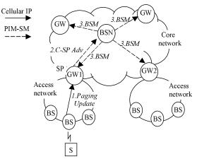
Fig. 4 Overview of SMM Proc. 1: The S transmits its multicast group and location to GW1 using a Paging Update message. GW1 becomes the source point for the group and sends an C-SP Adv message to BSN. The BSN broadcast BSM messages to all GWs.
