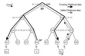
Fig. 11 SMM-A Proc. of handover of receiving member: R2 is moving to B7 cell. R2 sends *Enroll* message to N3 via N7. N7 has no MFCE for G, then, it creates  $E_{\rm G}({\rm N7}) = \{1, -1, 0\}$ . N3 already has MFCE for G, then, it update to  $E_{\rm G}({\rm N3}) = \{1, -1, -1\}$ .  $E_{\rm G}({\rm N6})$  is removed by timer or *Leave* message.
