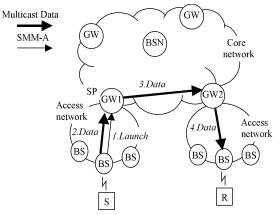
Fig. 6 Overview of SMM Proc. 3: Upon receiving the Page message, the S replies to GW1 with Launch message to create forwarding cache entries between the S and GW1. The S starts sending multicast data, and the data are forwarded to GW1, GW2 and R.
