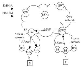
Fig. 5 Overview of SMM Proc. 2: The R sends an Enroll message for the multicast group to GW2 to create forwarding cache entries between the R and GW2 (SP). GW2 sends Join message to GW1. GW1, if it has not received multicast data, sends Page message to all BSs.
