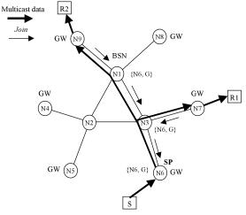
Fig. 15 SMM-C Proc. of source handover (3): The BSN floods BSM message to notify that N6 is the SP for G. N7 and N9 send a Join message to N6, thus a new SPT is constructed. N6 stops tunneling to N5.
