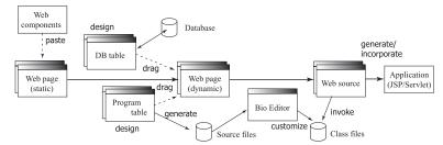
Fig. 1 Visual design and programming of Web applications.
