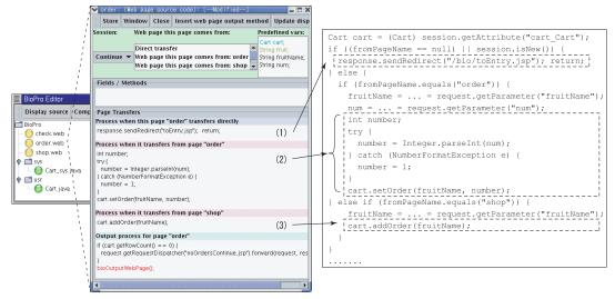
Fig. 6 Web source window for the "order" page and automatic code generation.
