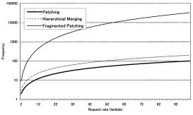
Fig. 16 Comparison of the frequency of multicast tree grafting for each technique.
