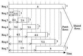
Fig. 6 Trunk link flows with the patching technique.
