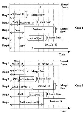
$\label{eq:Fig.9} Flows \mbox{ of the hierarchical merging technique on a branch.}$
