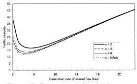
Fig. 11 Traffic intensity on a branch link, m = 2, with the hierarchical merging technique.
