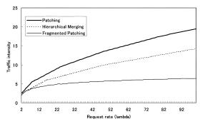
Fig. 14 Comparison of minimized traffic intensity on the trunk link for each technique.
