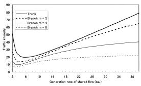
Fig. 10 Traffic intensity on each link with the patching technique.
