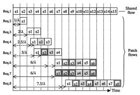
Fig. 4 Fragmented patching technique: requests arrive at random. The segments with a double box are those that differ from the segments in Fig. 3.
