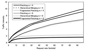
Fig. 15 Comparison of minimized traffic intensity on the branch links (m = 4 and 8) for each technique.
