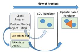
Fig. 3 Work flow of current implementationl
