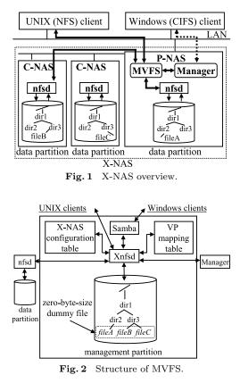
virtualized file system, MVFS for short, and a manager. MVFS virtualizes many data partitions as a unified one and distributes each file entity to one of the data partitions. The manager is responsible for manageability features such as on-line reconfiguration, autonomous rebalancing, and automatic migration facilities (Section 2.3).
