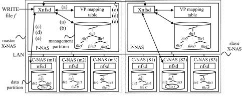
Fig. 6 Flow of WRITE operation on RX-NAS.
