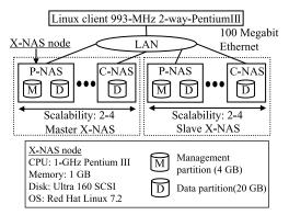
Fig. 10 Experimental environment of RX-NAS.
