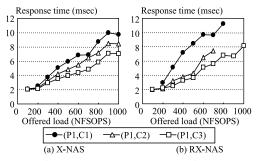
Fig. 16 Average response time for READ operations in the case of X-NAS and RX-NAS.
