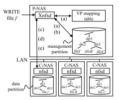
Fig. 4 Flow of WRITE operation.
