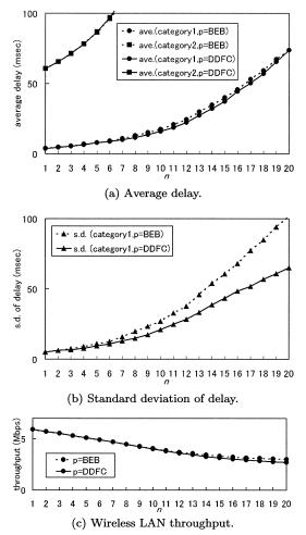
Fig. 6 The characteristics of EDCA. The parameter settings of the LAN are shown in Table 4, and EDCA settings are shown in Table 5. p is the backoff algorithm used by category 1 and n is the number of category 1 flows.  $t_s = 20 \text{ ms}$  and  $t_0 = 100 \text{ ms}$ .
