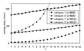
Fig. 2 The average delay characteristics in the differentiation framework of EDCA. The parameter settings of the LAN are shown in Table 4, and EDCA settings are shown in Table 3. p is the backoff algorithm used by category 1 and n is the number of category 1 flows.
