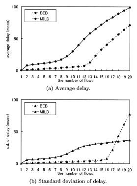
Fig. 1 The delay characteristics of BEB and MILD. The parameter settings of the LAN are shown in Table 4, and  $CW_{min}$  and  $CW_{max}$  are 31 and 1023 respectively. The bit rate of a flow is 192 kbps, the packet size is 512 B, and the queue length is 4 frames.
