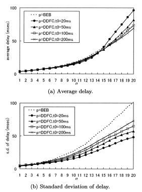
Fig. 7 The delay characteristics of category 1 traffic. The parameter settings of the LAN are shown in Table 4, and EDCA settings are shown in Table 5. p is the backoff algorithm used by category 1 and n is the number of category 1 flows.  $t_s = 20$  ms.
