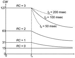
(b) Contention window controlled by DDFC.  $t_s$  and  $t_0$  are DDFC's protocol parameters.
