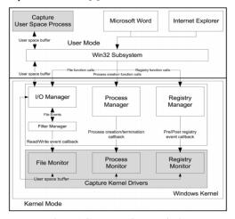
Figure-1 CaptureBat Structure in the system
