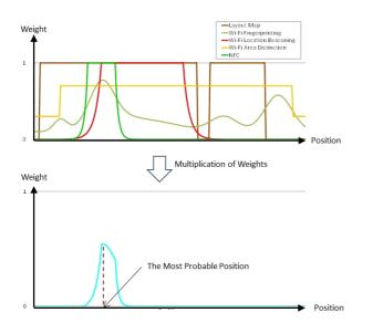
Fig. 7 Theory of Weighting for the Particle Filter
