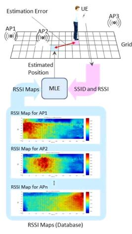
Fig. 2 Wi-Fi Fingerprinting
