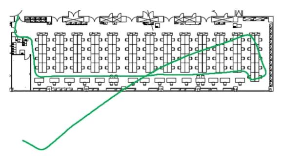
${\bf Fig. \ 12} \quad {\rm A \ Sample \ of \ Trajectory \ Path \ Estimated \ Using \ the \ PDR}$
