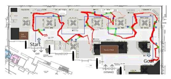
Fig. 16 A Sample of Trajectory Path Estimated by Combining PDR, Wi-Fi Fingerprint, Layout Map, Wi-Fi Location Beacon and NFC
