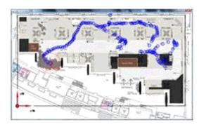
Fig. 20 Trajectory Path Estimated Using a 6m Grid Size RSSI Map
