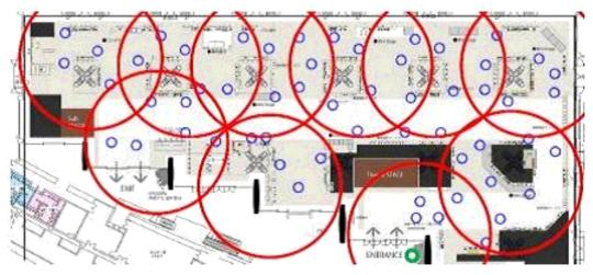
Fig. 14 Arrangement of AP, Location Beacon and NFC
