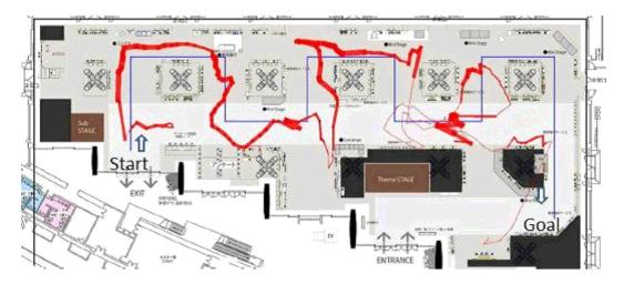
Fig. 15 A Sample of Trajectory Path Estimated by Combining PDR, Wi-Fi Fingerprint and Layout Map
