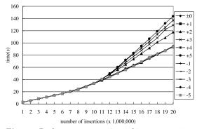
**Fig. 12** Performance comparison of insert operations with varying d.
