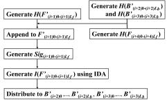
Fig. 6 Signature method of F packets.
