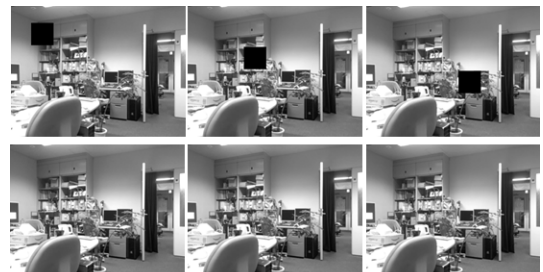
Fig. 4 Results of inpainting on 'room' sequence. Top row: masked input. Bottom row: inpainted output.
