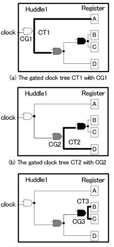
(c) The gated clock tree CT3 with CG3 Fig. 3 Three-stage clock tree in a huddle.
