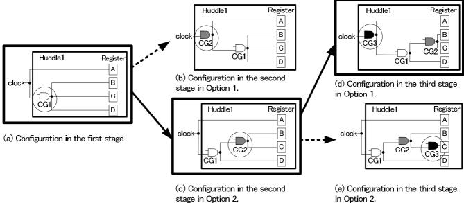
Fig. 6 Clock tree configurations associated with Fig. 5.
