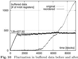
Fig. 10 Fluctuation in buffered data before and after test vector reordering for s9234.
