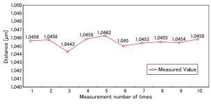
Fig. 7 Result of measurement accuracy examination
