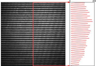
Fig. 4 Single interference fringe of a flat mirror.
