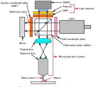
Fig. 1 Structure of proposed 3D microscope.
