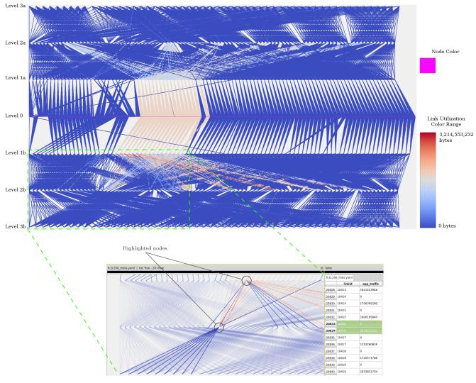
Fig. 3 A BoxFish visualization of the NPB FT benchmark running on 256 nodes of TSUBAME2.5 with the class D problem size. The upper image shows the full view of the network while the lower image shows a close-up of the most utilized link being highlighted.
