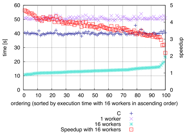
Fig. 14 Execution time and speedup with 16 workers versus vertex ordering (sorted by execution time with 16 workers).
