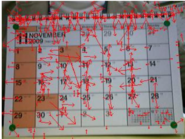
Fig. 2 Example of interest points, scales and their principal directions detected by SIFT.
