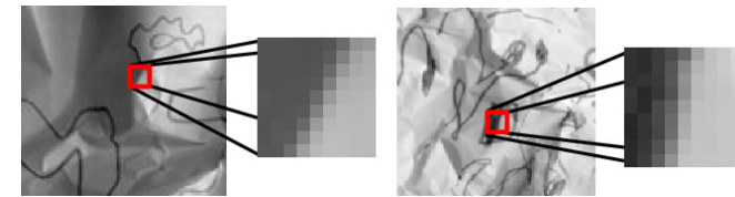
Fig. 5 These images show how a system based on using only patches of data can encounter difficult ambiguities. The two enlarged patches look very similar, but one patch comes from an edge caused by a change in albedo, while the other comes from a change in shading.
