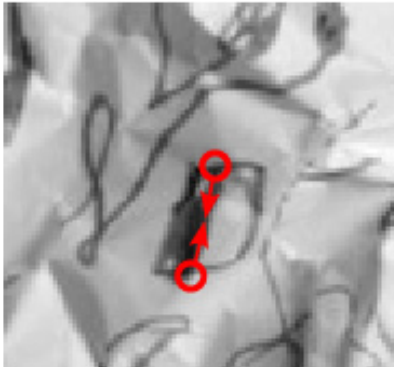
Fig. 6 Using only local information, the vertical edge at the center of the image could be viewed as either a painted line or a sharp fold in the surface. However, if information is propagated from the regions highlighted with circles along the edges, then the classification can be disambiguated.
