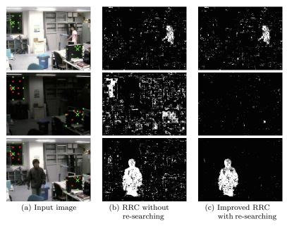
Fig. 4 Effect of our improved RRC. Green and red marks in the input images show typical examples of peripheral pixels which are sought again: green crosses are center pixels, red dots are their initial peripheral pixels, and green dots are peripheral pixels which are found in the re-searching process.
