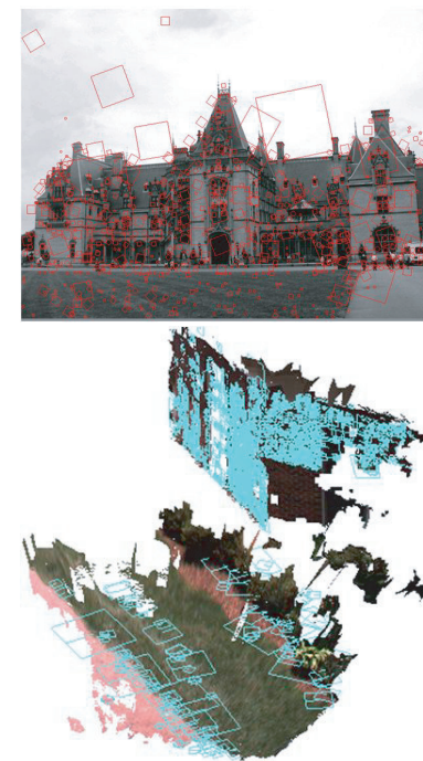
Fig. 13 While SIFT features are extracted from 2D images and are not fully invariant to viewpoint (left), VIP features are extracted on the 3D surface which provide viewpoint invariance and enables single match hypotheses (right).
