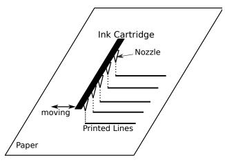
Figure 1: Inkjet printing mechanism
