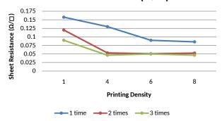
Figure 5: Change of sheet resistance depends on Density and Overprinting time
