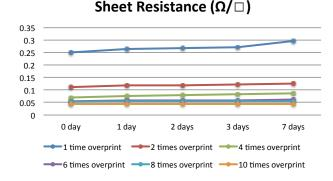
Figure 4: Change of sheet resistance after several days
