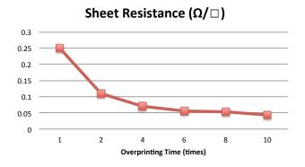
Figure 3: Change of sheet resistance depends on number of overprinting time
