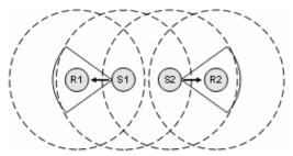
Fig. 2 Directional antenna resolves exposed terminal problem.
