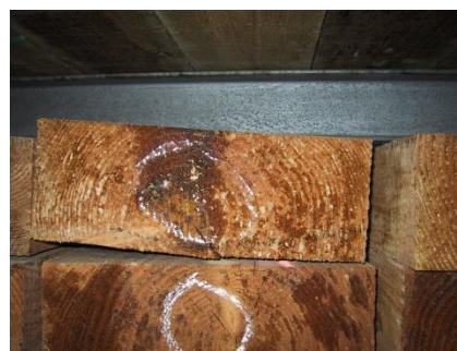
図13 乾燥後の木材の反りと年輪[2] Figure13 Wood Warpage and Annual Growth Ring
