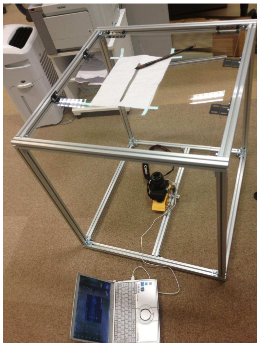
Fig. 1 Illustration of our footprint capturing device.
