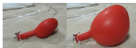
(a)収縮時の様子 (b)膨張時の様子 (a) Contracted state (b) Expanded state
