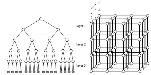
**Fig. 5** Embedding a 63-node complete binary tree into  $M(4, 4, 4)$ . Subtrees in layer 1, 2, and 3 are mapped on 1-dimensional grids along  $x$ -,  $y$ -,  $z$ -axis, respectively.
