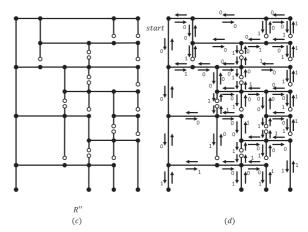
Fig. 3 (a) A rectangular drawing R, (b) removal of the botttommost horizontal line segment, (c) replacement of lower right corners, (d) the trace.
