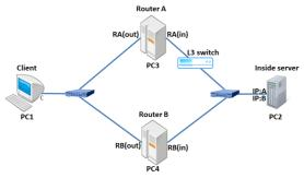
Fig. 8 Evaluation network configuration with L3 switch.
