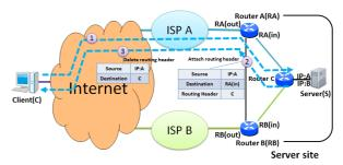
Fig. 4 Route control using the routing header.
