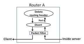
Fig. 6 Site-exit router configuration.
